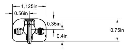
If the template is printed to scale, the distance between the two lines will measure 3/4".
